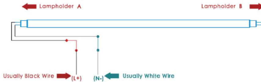
Figure 6: After retrofit – Rewiring the wires from Lampholder A to “L” and “N” of the supply circuit by wire nuts/connectors. Insulated or capped all unused conductors with a wire connectors.
